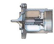
Release with a tensile force being applied at an angle to the plane of the coupling housing, up to 90 degrees.
